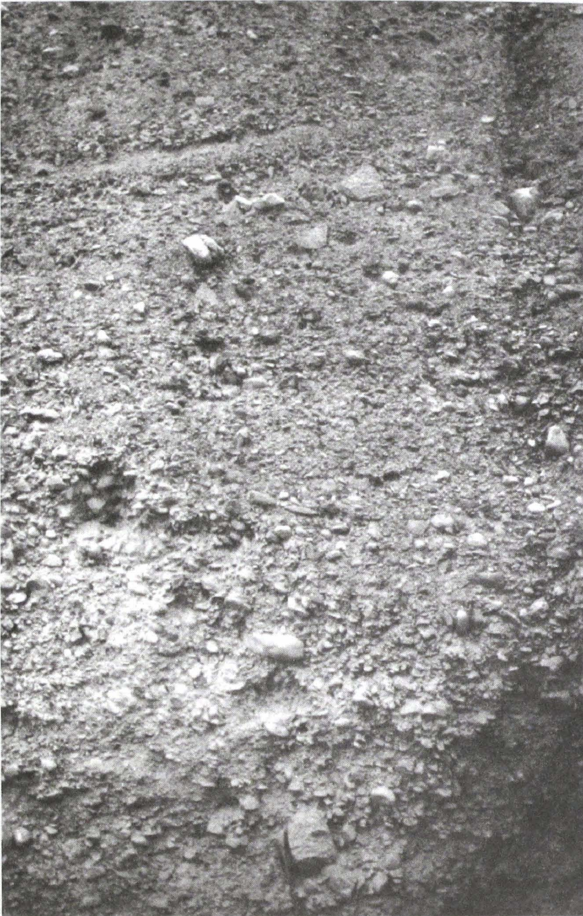
6. Exposed section of the conglomerate showing the composition with gravels.
